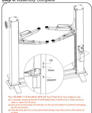
Be sure to turn the lift off when not in use to prevent damaging the batteries
