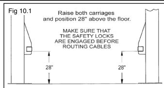
2. With the carriages locked at 28" off the floor, route the threaded end of the equalizer cable across to the opposite side base plate sheave and up through the carriage. (See Fig. 10.2)
