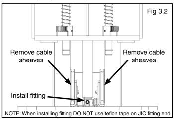
3. Route button end of the cable upwards through the bottom of the carriage and wrap the cable around the cable sheave and reinstall sheave by reversing the sheave removal procedure. Leave excess cable tied together in a coil to carriage until further steps are required. (See Fig 3.3 & 3.4)
