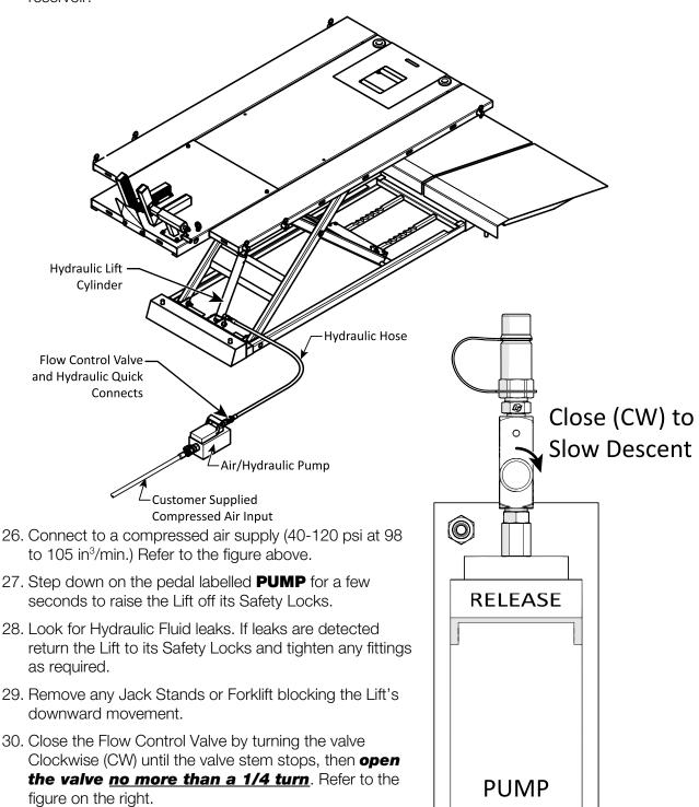
**WARNING!** Failure to close the Flow Control Valve may result in rapid platform descent and possible severe injury.
