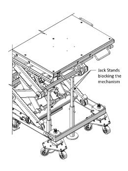
b. After raising the top deck to rest on the third safety lock, use jack stands or an equivalent, as detailed above, to ensure the safety of personnel and stability of the Lift while working under it.
