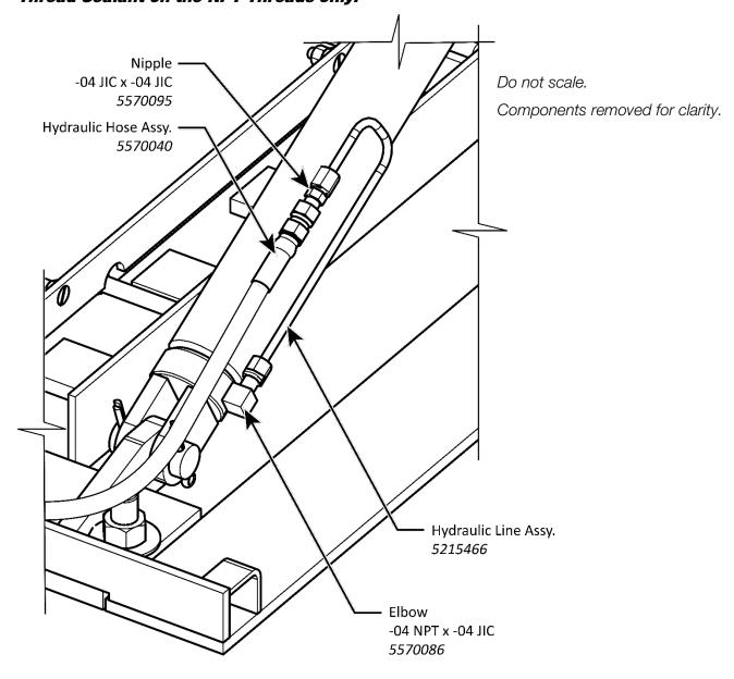
6. Attach the Straight End of the Hydraulic Line Assembly (5215466) to the Hydraulic Elbow Fitting you just attached, then attach a Nipple (5570095) to the end of the Hydraulic Line.
