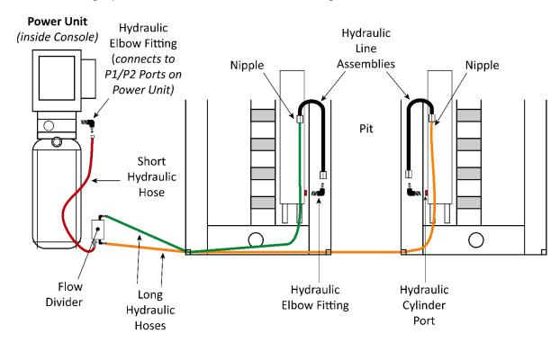
Fittings shown not connected for clarity. Drawing not to scale.
