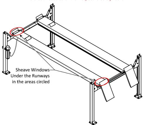
3. Note the Lift Cable's top or bottom Sheave position. The Lift Cables must be returned to their original position. Working under the Powerside Ramp, remove the Two Sheaves on the Cylinder Side. Set the Sheaves and their Pin aside where they will not be damaged.
