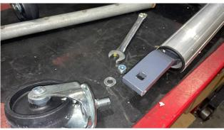
2. Examine the outside diameter of the Roller Guard. It consists of a plastic ring with a step reducing down to a smaller outside diameter. Slide the Guard's small diameter side over the Frame and *carefully* snap the Guard into the Aluminum Roller. Lift the Aluminum Roller up and away from the Jack Frame and slowly apply pressure to the Roller Guard until it snaps in. Refer to the image on the next page.
