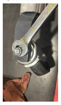
4. Verify the casters are secure and the Aluminum Rollers rotate freely without binding.
