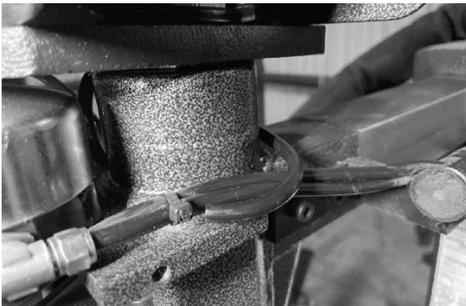
5. Attach one end of the Tee Compression Fitting (5550395) to the Bead Lifter Air Line, then connect both ends of the split Air Line to the Tee Compression Fitting. Verify the connections are properly secured.
