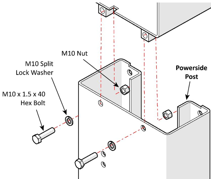
3. Align the holes on the top of the Offside Post with the holes on the bottom of the Top Trough, then connect the two using the supplied 10 mm hex bolts, washers, and nuts.
