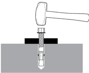
The Expansion Sleeve of the Anchor Bolt may prevent the Anchor Bolt from passing through the hole in the Base Plate; this is normal. Use a hammer or mallet to get the Expansion Sleeve through the Base Plate and into the hole.
