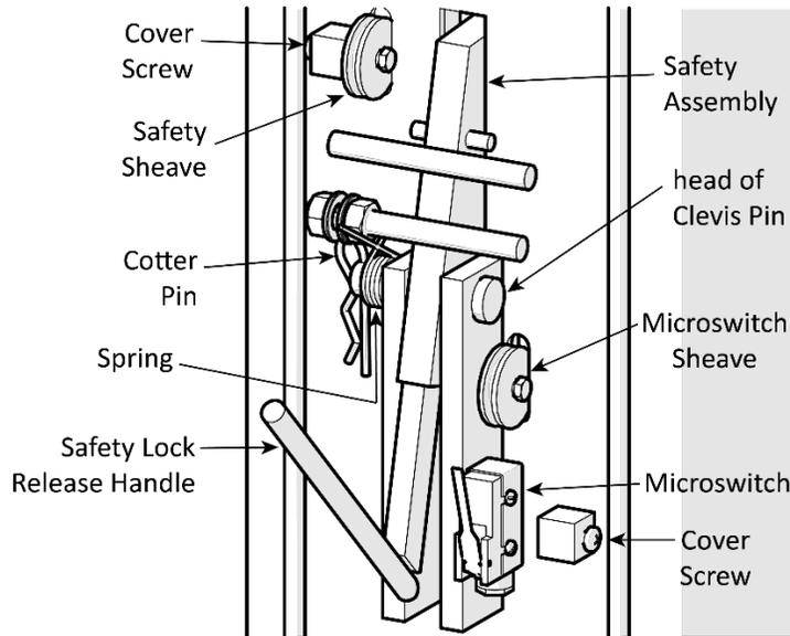
The following drawing shows the components of the **Offside** Safety Assembly.
