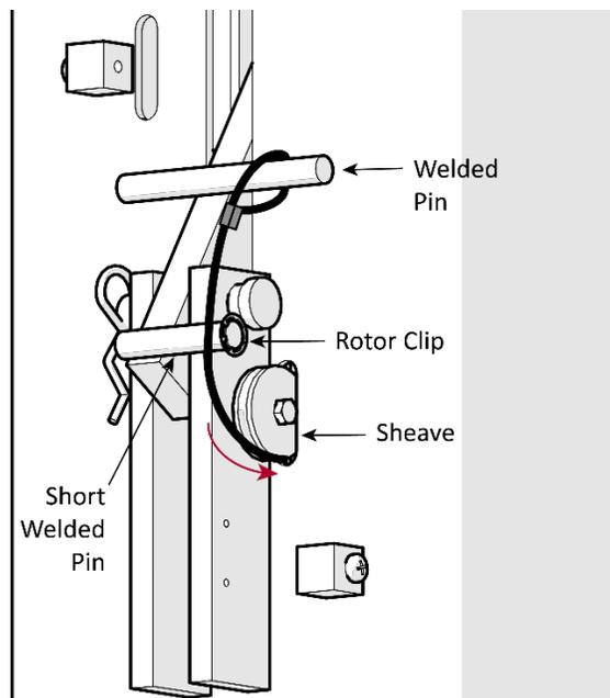
4. On the **Powerside Post**, screw two Nuts onto the threaded end of the Welded Pin with Threads. Make sure that one is on each side of the hole in the Welded Pin with Threads.
