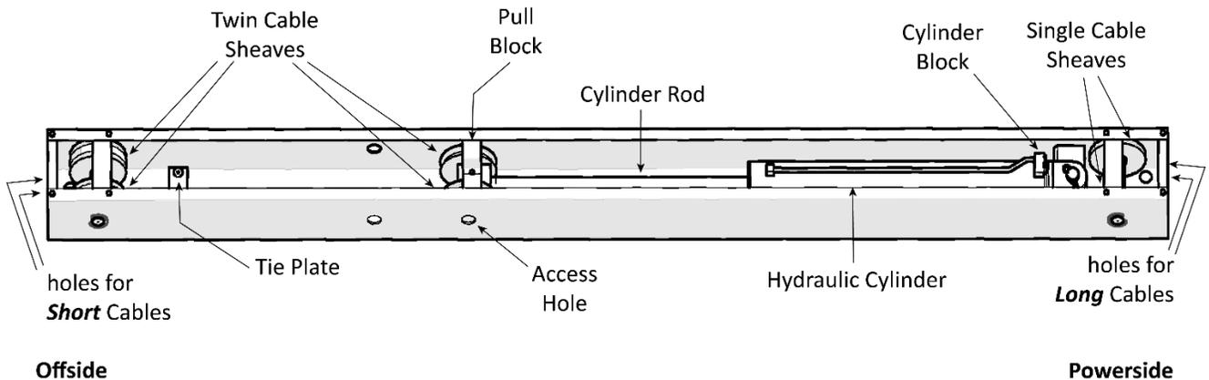
*Not all components shown. Tie Plate and holes for Cables not visible from side view of Top Trough.*
