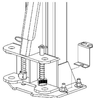
9. ***Do not torque the Anchor Bolts at this point.***
