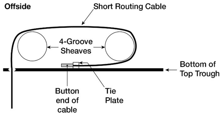
3. Route the Short Cable under the bottom of the Cylinder sheave and then over the top of it, over the top of the Offside end sheave, and down through the hole in the bottom of the Top Trough.
