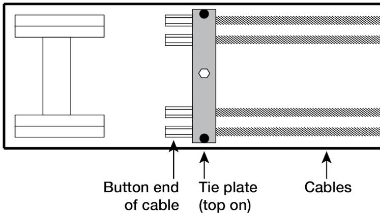
**Important:** Make sure the cables are carefully aligned in their sheaves; you want to avoid as much contact as possible between the cable and the sheaves while the Lift is in motion. This makes the Lift move more smoothly and extends the life of the cables and the sheaves.
