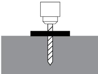
Do not drill all the way through the Concrete; if you punch completely through the slab, you could compromise the holding strength of the Anchor Bolts.
