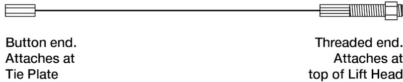
The Button end of all four cables **start** at the same place at the Tie Plate, in the Top Trough.
