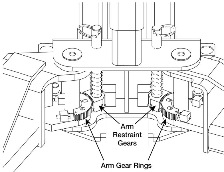
**Important:** Arm Gear Rings have a Left or Right orientation, based on looking at the Post from the inside of the Lift, as shown above. You must correctly orient the arms.
