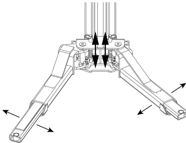
Make sure the Lift Arms do not move when a force of approximately 100 pounds or less is applied laterally to the fully extended arms.
