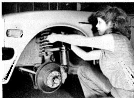
Hold Spring Pak by top arms and spread them over highest accessible coil. Arms are spring loaded to hold them in place during mounting on spring.
