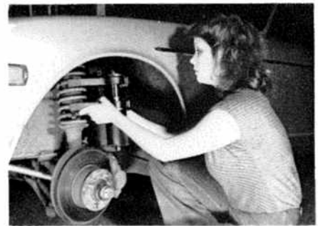
Spread lower Spring Pak arms and attach to lowest possible coil. Again, spring loading holds arms and unit in place on coil.
