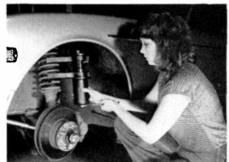
Using ratchet or wrench, turn nut at bottom of Spring Pak, compressing coil spring. Position safety pin, disconnect strut at top and remove Spring Pak and coil spring as a unit. It's just that simple.
