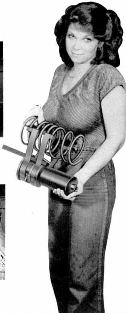
Hold Spring Pak by top arms and spread them over highest accessible coil. Arms are spring loaded to hold them in place during mounting on spring.
